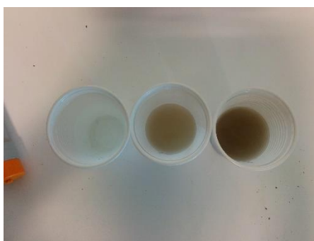
Figure 2: Water colour in System 1 (left), System 2 (center), and System 3 (right) immediately after the addition of wood ash in Systems 2 and 3.
