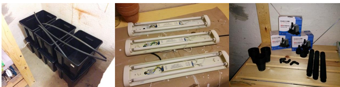
Figure 5: From left to right: The three container units with the plumbing tubes, the three light fixtures, and the three pumps, connectors, standpipes, and bulkhead fittings.
