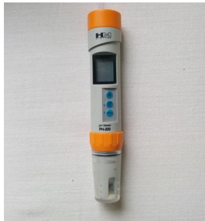
Figure 1: HM Digital waterproof PH-200 used for measuring the pH of the collected urine.
