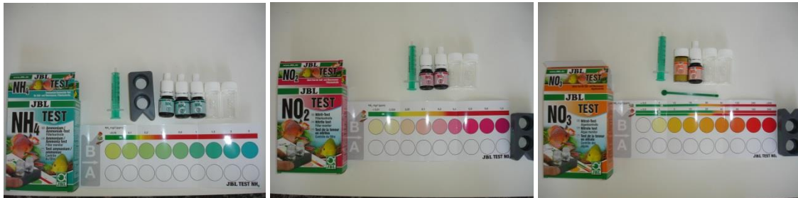
Figure 2: From left to right: JBL test kits for Ammonium/Ammonia, Nitrite and Nitrate.
