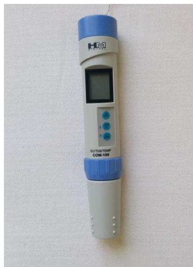
Figure 3: HM Digital waterproof COM-100 used for measuring the EC of the systems' water.
