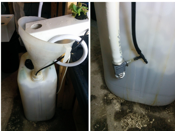
Close-up of the NFT anthroponics system's MBBR (left) and the airlift system out of the MBBR for inspection (right). Photos taken by the author in Malmö, Sweden in 2017.
